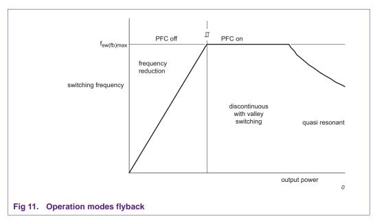
At maximum output power, limited by the flyback current sense resistor, the flyback controller operates in Quasi-Resonant (QR) mode. The next primary switching cycle starts at detection of the first valley.
