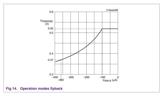
The total OPP resistance determines the  $I_{FBAUX}$  current during the primary stroke of the flyback and consists of R23 + R23A (see <u>Figure 13</u>). First, the OVP resistor R23 has to be calculated before the remaining part of the OPP resistor R23A can be calculated.
