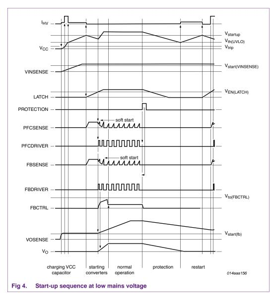
The charge time of the soft-start capacitors is set by choosing their values independently for the PFC and the flyback controller. In this way, it can be realized that the PFC starts before the flyback.
