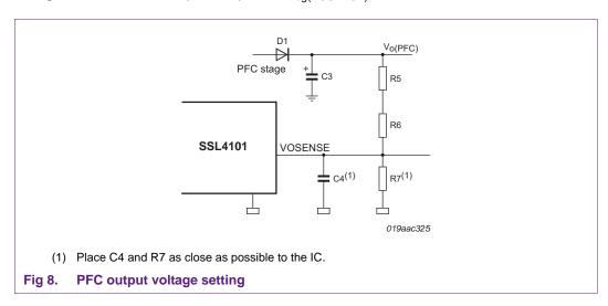
Two resistors of 4.7 M $\Omega$  (1 %) can be used for low no-load input power placed between the bulk elcap and the VOSENSE pin. With a resistor value of 4.7 M $\Omega$  for R5 and R6 and 60 k $\Omega$  to 62 k $\Omega$  for R7, a universal mains adapter will have a PFC output voltage of approximately 380 V to 390 V at high mains and 240 V to 250 V at low mains.
