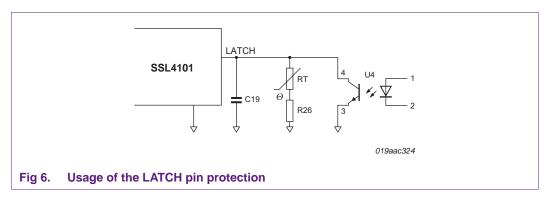
Latching on application overtemperature occurs when the total resistance value of the Negative Temperature Coefficient (NTC) and its series resistor drops below the following:
