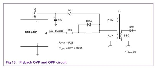
At a current  $I_{ovp(FBAUX)}$  of 300  $\mu A$  on the FBAUX pin, the IC detects an overvoltage. An internal integrator filters noise and voltage spikes. The output of the integrator is used as an input for an up-down counter. The counter has been added as an extra filter to prevent false OVP detection which might occur during ESD or lightning events.
